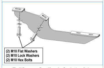
(Fig 2) Passenger Front Mounting Bracket Installation
