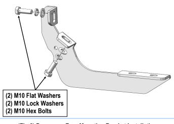
(Fig 6) Passenger Rear Mounting Bracket Installation
