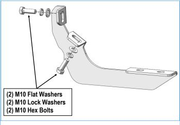
(Fig 4) Passenger Side Center Mounting Brackets Installation
