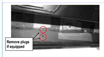
(Fig 3) Passenger Side Center Mounting Location
