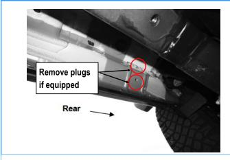
(Fig 5) Passenger Side Rear Mounting Location
