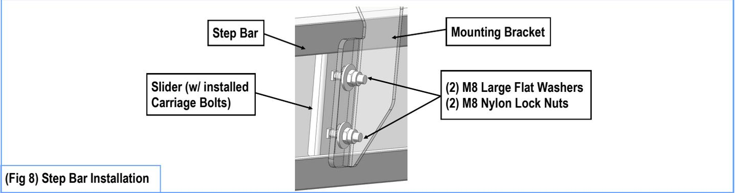
(Fig 8) Step Bar Installation
