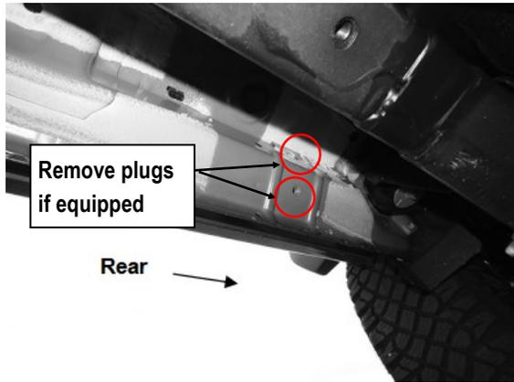
(Fig 5) Passenger Side Rear Mounting Location
