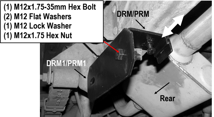
(Fig 6) Passenger Rear Mounting Bracket 1 Installed
