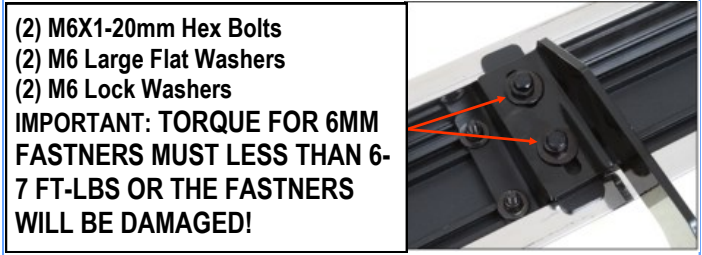
(Fig 14) Step Bar Installed on Bracket Installed (Example)
