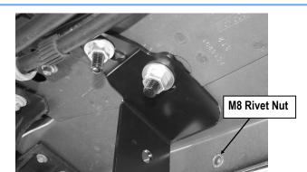
(Fig 15) M8 Rivet Nut Installed on Pinch Weld (Driver Rear Support Bracket Location)
