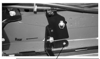
Mark and drill a 7/16" hole on pinch weld according to the location of Support Bracket
