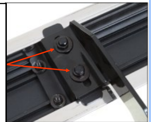
(Fig 19) Step Bar Installed on Bracket Installed (Example)
