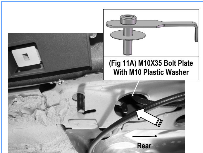
(Fig 11) Insert 10mm Bolt Plate Installation (On Driver Side Rear Mounting Location)
