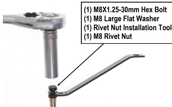
(Fig 7A) Assemble the Rivet Nut Installation Tool
