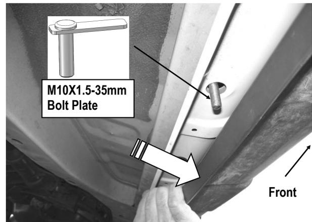
(Fig 3) M10 Bolt Plate Installed
