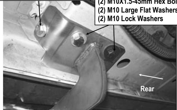
(Fig 10) Driver Rear Mounting Bracket (DRM) Installed
