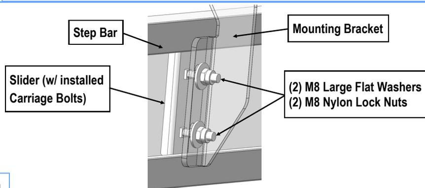
(Fig 13) Step Bar Installation
