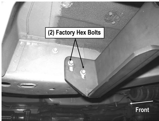
(Fig 5) Driver Front Mounting Bracket (DFM) Installed
