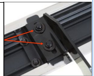
(Fig 11) Step Bar Installed on Bracket Installed (Example)
