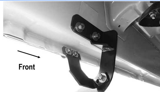
(Fig 15) Driver Side 2nd Brackets Installed
