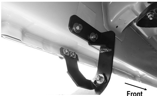
(Fig 14) Driver Side Front Brackets Installed
