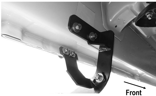
(Fig 14) Driver Side Front Brackets Installed (Example)
