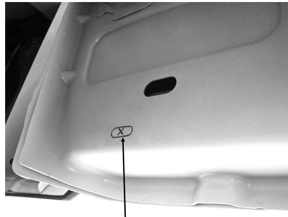
(Fig 20) Use A 7/16" Drill Bit To Drill Hole In Center Of Slot As Marked
