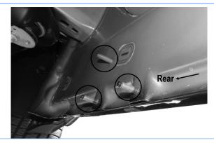
(Fig 7) Driver Side Rear Mounting Location
