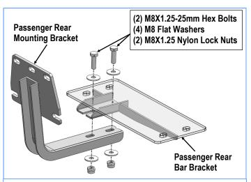
(Fig 8) Passenger Rear Bar Bracket and Passenger Rear Mounting Bracket Assembly
