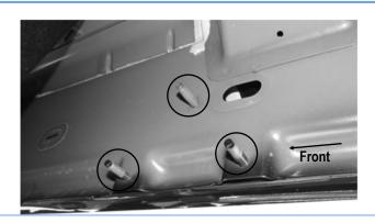
(Fig 4) Passenger Side Mounting Location
