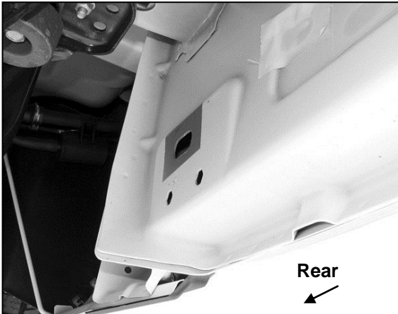
(Fig 15) Driver/Left 3# mounting location
