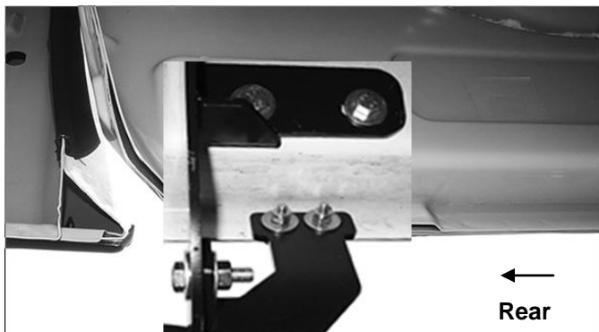
(Fig 16) Driver/Left rear upper Mounting Bracket assembly
