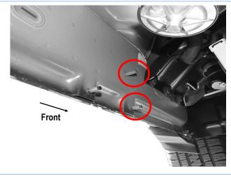
(Fig 1) Driver Side Front Mounting Location
