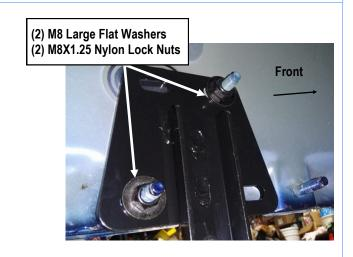
(Fig 3) Driver Center Mounting Bracket Installed
