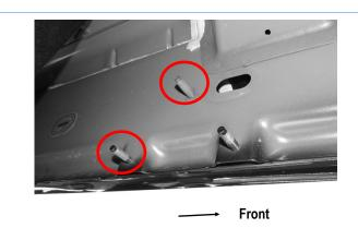
(Fig 2) Driver Side Center Mounting Location
