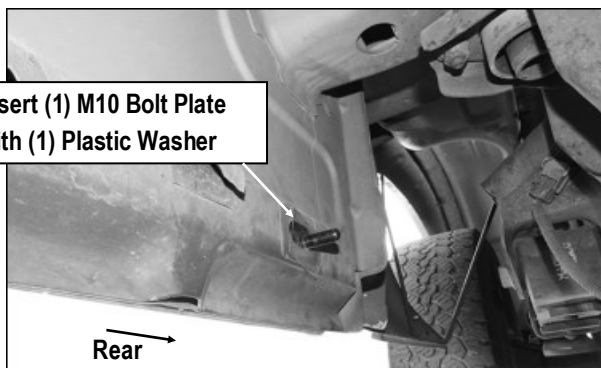
(Fig 8) Insert M10 Bolt Plate with (1) M10 Plastic Washer ( on Passenger Side Rear Mounting Location )
