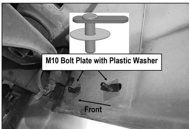
(Fig 2) M10 Bolt Plates with M10 Plastic Washers
