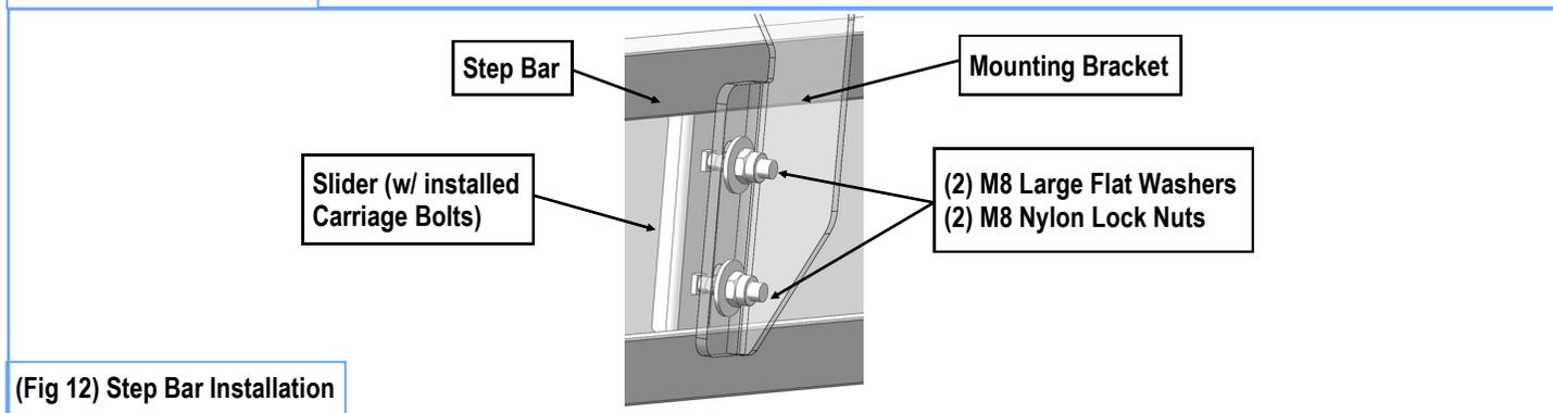
(Fig 12) Step Bar Installation
