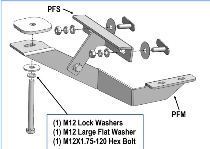
(Fig 4) Passenger Front Mounting Bracket Installation
