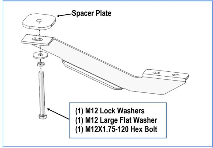
(Fig 6) Passenger Side Center Mounting Bracket Installation
