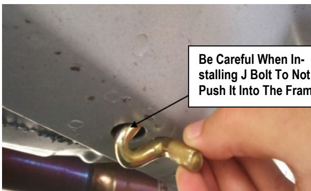
(Fig 2) Insert The M10X1.5 J-Bolt
