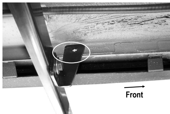
(Fig 13) Mark The Locations Onto The Inner Side Of The Pinch Weld
