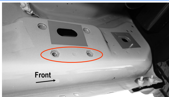
(Fig 7) Driver Side Front Mounting Location (Mid 2015-On, An Example Of Models With Factory Installed Threaded Inserts)
