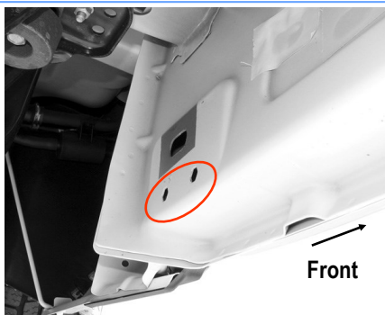
(Fig 11) Driver Side Rear Mounting Location
