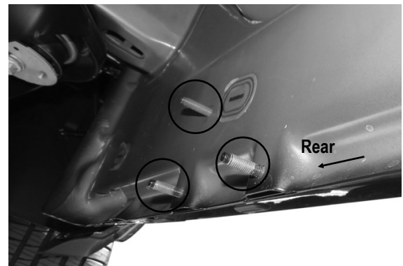
(Fig 4) Driver Side Rear Mounting Location
