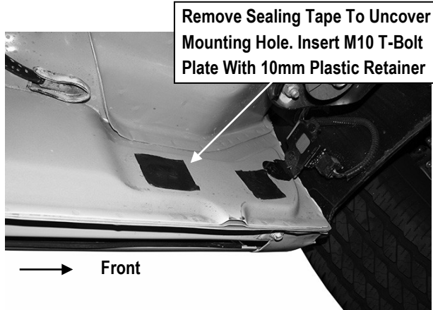
(Fig 1) Driver Front Mounting Bracket (DFM/DRM) Location
