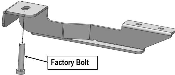
(Fig 1) Driver Front Mounting Bracket Installation
