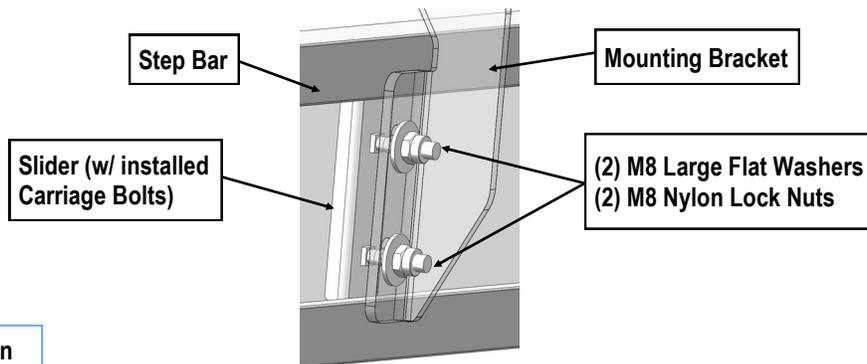
(Fig 3) Step Bar Installation
