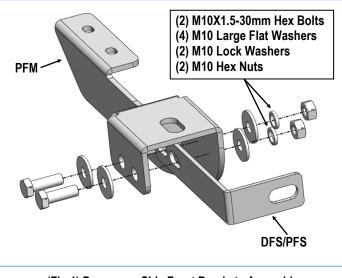
(Fig 1) Passenger Side Front Brackets Assembly
