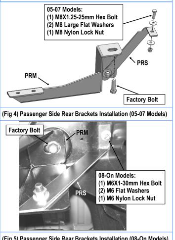
(Fig 5) Passenger Side Rear Brackets Installation (08-On Models)
