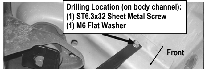
(Fig 4) Driver Front Support Bracket (DFS/PFS) Installation
