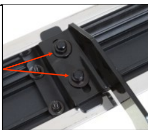
(Fig 15) Step Bar Installed on Bracket Installed (Example)
