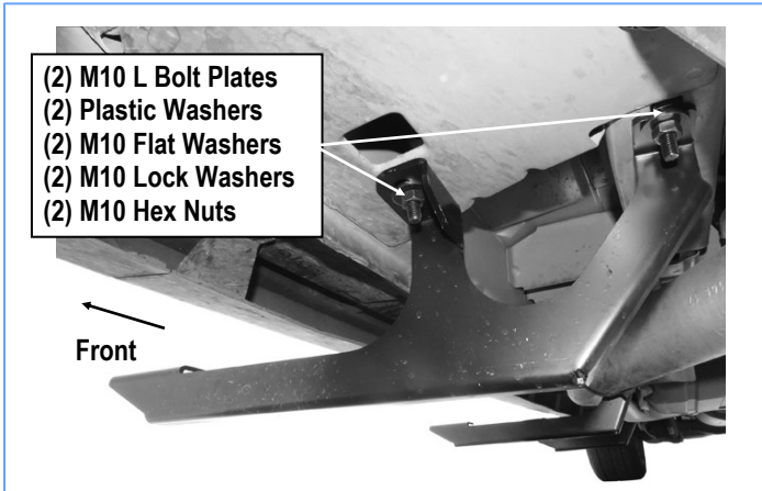
(Fig 4) Passenger Front Mounting Bracket Installed
