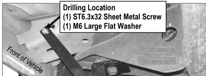
(Fig 7) Driver Side Rear Support Bracket (DRS/PRS) Installed
