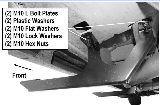
(Fig 4) Passenger Front Mounting Bracket Installed
