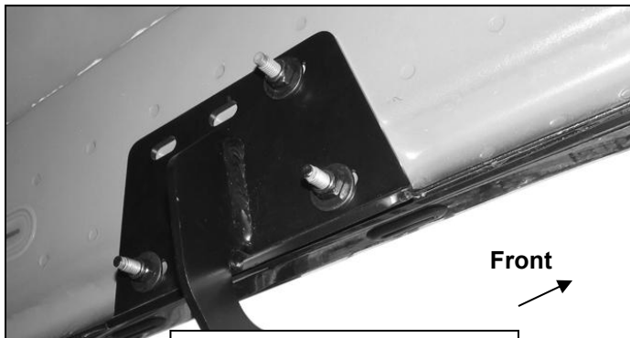
(Fig 3) Driver/left front side Mounting Bracket installed
