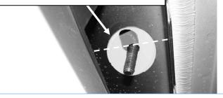
(Fig 4) M10 Bolt Plate Installed on Driver Side Front Mounting Location
