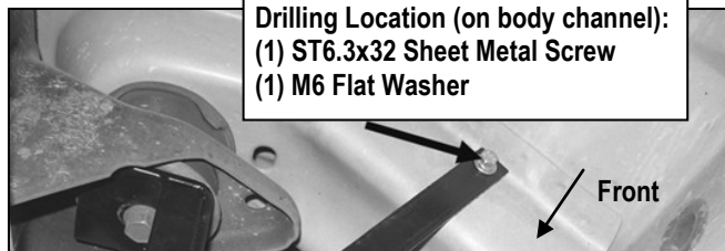
(Fig 4) Driver Front Support Bracket (DFS/PFS) Installation
