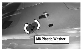
(Fig 5) Thread Plastic Washer onto Bolt Plate to hold Bolt Plate in position
