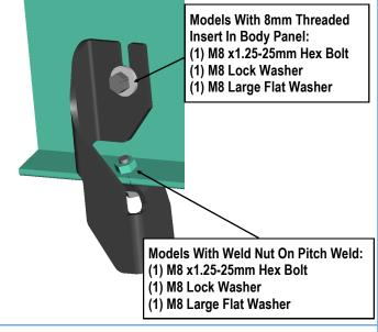
(Fig 18) Passenger Front Mounting Bracket Installation (Weld Nut If Equipped-Also See Fig 5)
