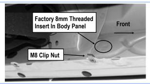
(Fig 6) Driver Side Center Mounting Location
