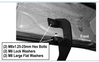
(Fig 9) Driver Front Mounting Bracket Installed
