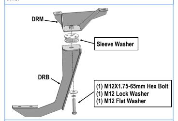
(Fig 11) Driver Rear Mounting Brackets Assembly
