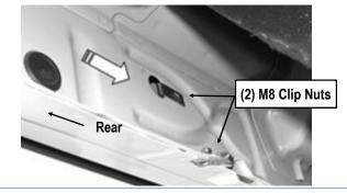
(Fig 8) Driver Side Rear Mounting Location
