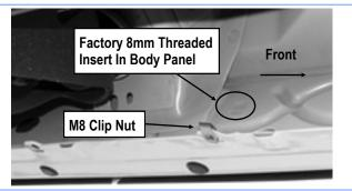
(Fig 6) Driver Side Center Mounting Location
