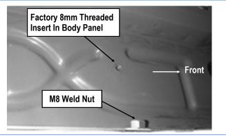
(Fig 5) Driver Front Mounting Bracket Location
