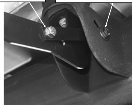
(Fig 7) Passenger Center Bracket Installed (Up to 2011 2500/3500 Models )
