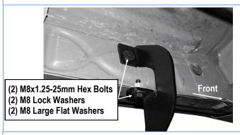
(Fig 9) Driver Front Mounting Bracket Installed
