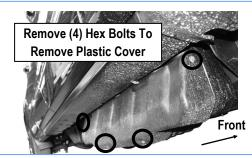
(Fig 14A) 2017-Up Passenger Side Pictured With DEF Plastic Tank Cover
