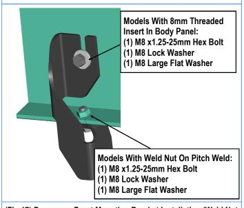
(Fig 17) Passenger Front Mounting Bracket Installation (Weld Nut If Equipped-Also See Fig 2)
