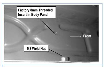
(Fig 5) Driver Side Front Mounting Location
