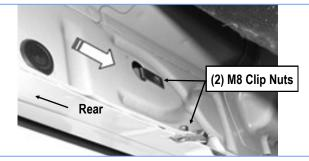
(Fig 8) Driver Side Rear Mounting Location
