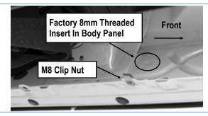
(Fig 6) Driver Side Center Mounting Location
