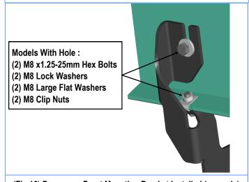
(Fig 16) Passenger Front Mounting Bracket Installed (example)
