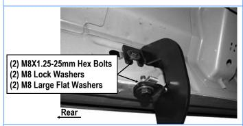
(Fig 10B) Assembled Driver Rear Mounting Bracket Installed
