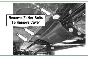
(Fig 13) 07-16 Passenger Side Front With DEF Tank Cover
