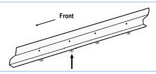
(Fig 18) Passenger 2nd Mounting Bracket Location From Back Of Body Panel
