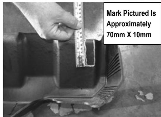
(Fig 19) 2017-Up Passenger Side DEF Cover Marked For Trimming
