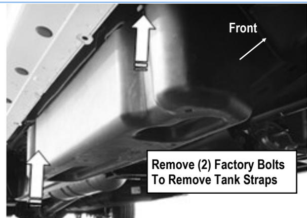
(Fig 15) 07-16 Passenger Side DEF Tank And Cover
