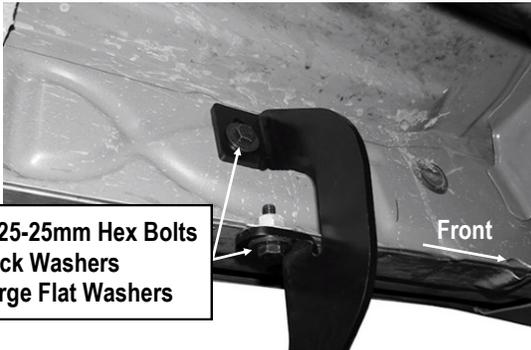
(Fig 9) Driver Front Mounting Bracket Installed
