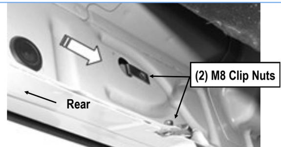
(Fig 8) Driver Side Rear Mounting Location
