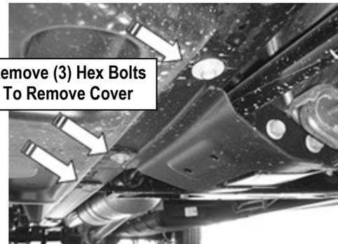
(Fig 13) 07-16 Passenger Side Front With DEF Tank Cover
