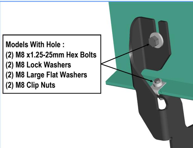
(Fig 16) Passenger Front Mounting Bracket Installed (example)
