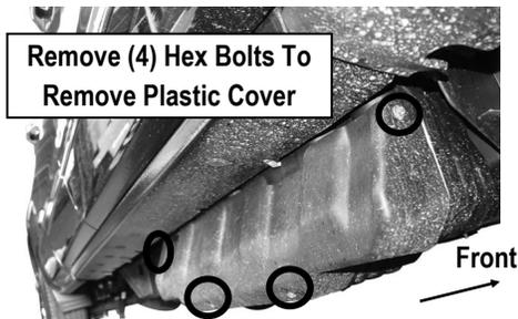
(Fig 14A) 2017-Up Passenger Side Pictured With DEF Plastic Tank Cover
