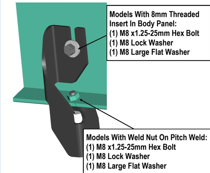
(Fig 17) Passenger Front Mounting Bracket Installation (Weld Nut If Equipped-Also See Fig 2)
