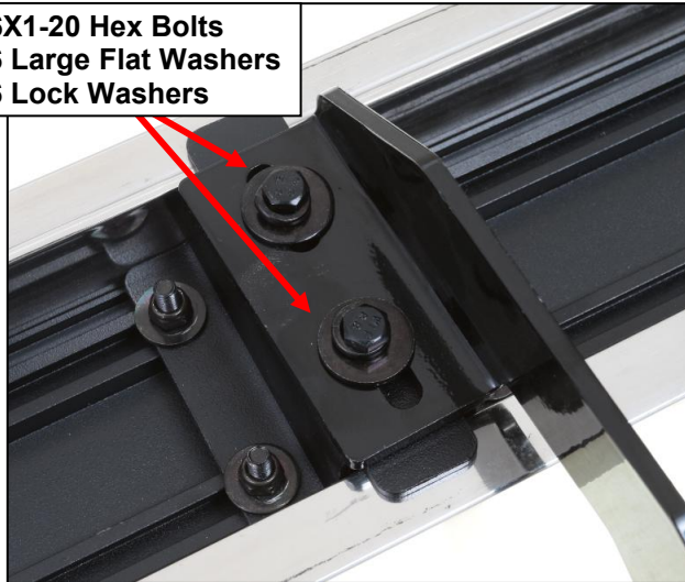
(Fig 7) Bracket Installation
