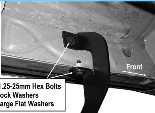
(Fig 9) Driver Front Mounting Bracket Installed
