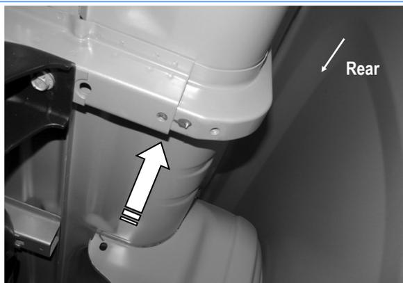
(Fig 13) Driver Rear Mounting Bracket Location
