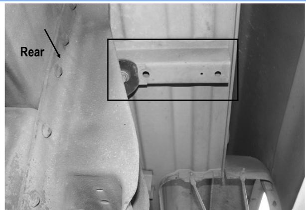
(Fig 10) Driver Rear Mounting Bracket Location
