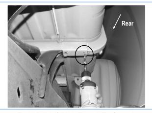
(Fig 14) Drill A 1/2" Hole Through The Channel
