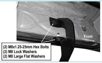
(Fig 9) Driver Front Mounting Bracket Installed
