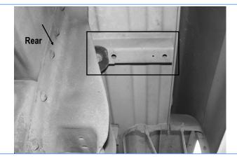
(Fig 10) Driver Rear Mounting Bracket Location (Early "Long" Bed Support)
