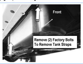
(Fig 22) 07-16 Passenger Side DEF Tank And Cover
