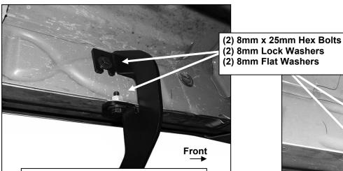
(Fig 6) Driver/left front bracket installed
