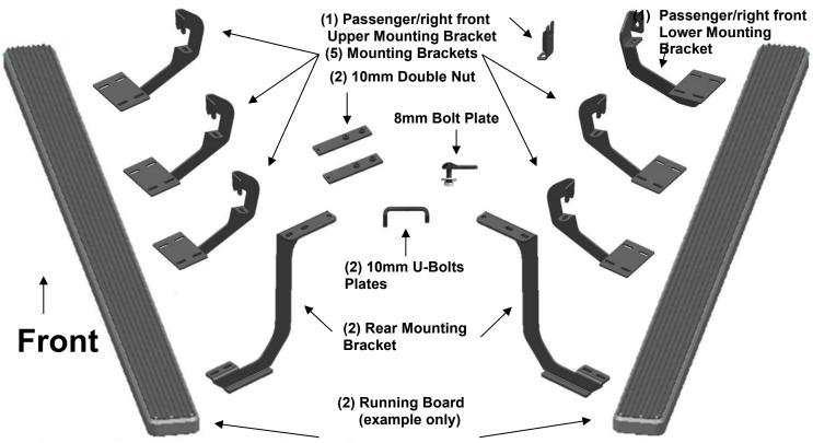
IMPORTANT ALERT: FOR WHEEL TO WHEEL APPLICATION, WEIGHT TO THE REAR END AREA OF THE RUNNING BOARD BEHIDE THE LAST BRACKET NEED TO LESS THEN 130KG.OVERWEIGHT IN THIS AREA MAYBE DAMAGE YOUR RUNNING BOARD.
