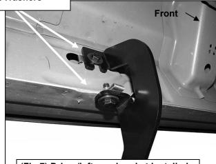
(Fig 7) Driver/left rear bracket installed
