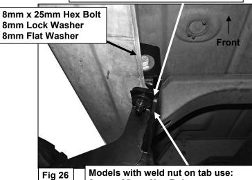
8mm x 25mm Hex Bolt 8mm Lock Washer 8mm Flat Washer
