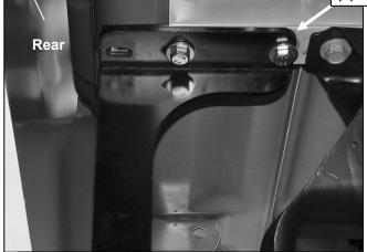
(Fig 14) Bolt Rear Bracket to Double Nut Plate
