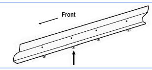
(Fig 19) Passenger 2nd Mounting Bracket Location From Back Of Body Panel
