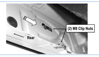
(Fig 8) Driver Side Rear Mounting Location
