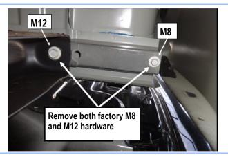
(Fig 10A) Driver Side Rear Mounting Location
