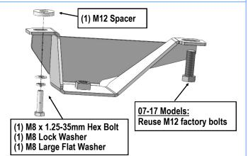
(Fig 10B) Driver Rear Mounting Bracket Installation
