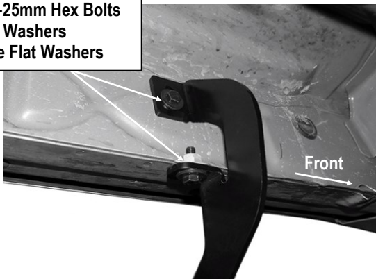
(Fig 6) Driver Front Mounting Bracket Installed
