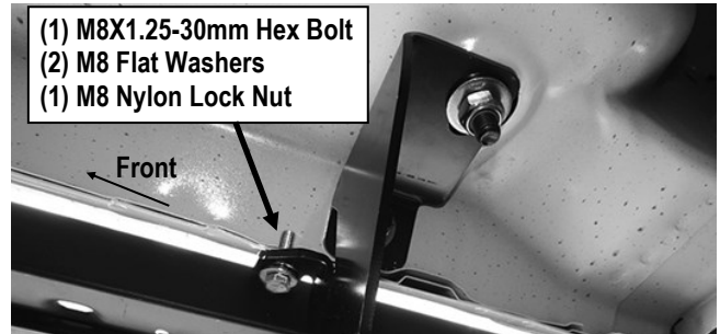
(Fig 17) Passenger Center Mounting Bracket Attached to the Pinch Weld
