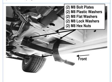
(Fig 3) Passenger Side Front Brackets Installed
