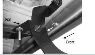
(Fig 9) Passenger Side Center Brackets Installed
