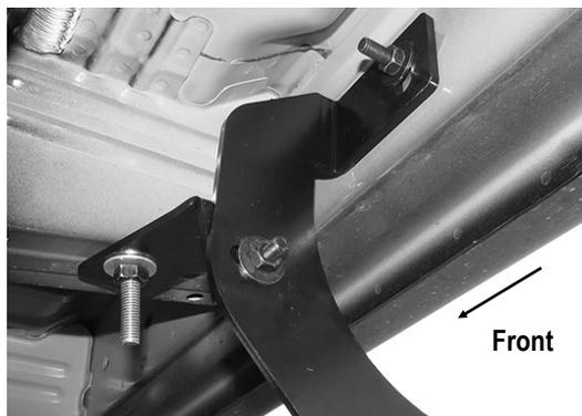
(Fig 9) Passenger Side Center Brackets Installed
