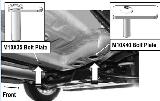
(Fig 1) Insert The M10 Bolt Plates
