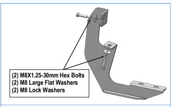
(Fig 2) Passenger Front Mounting Bracket Installation
