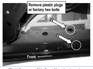
(Fig 1) Passenger Side Front Mounting Location
