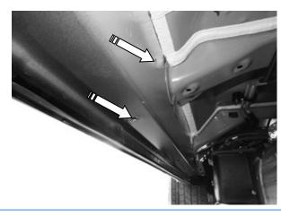
(Fig 4) Passenger 3rd Mounting Bracket Location
